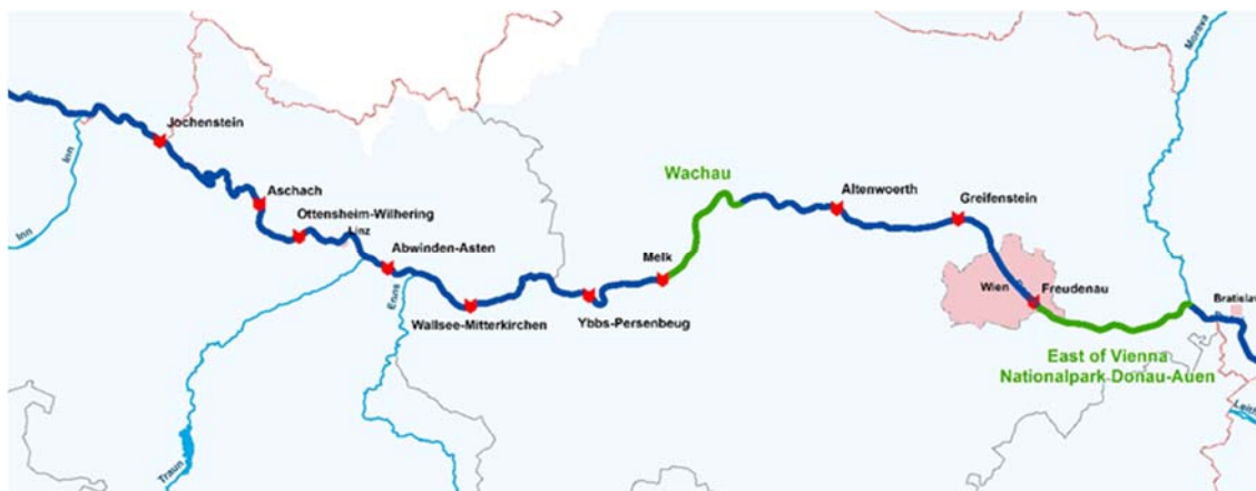
Figure 24: The Danube River in Austria: Locations of the hydropower plants (red) and the free-flowing sections (green) (bed levels: VHP and viadonau; water levels and locations of the hydropower plants: viadonau (2012)).
